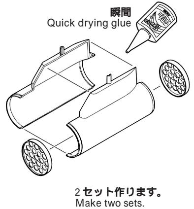
Assemble the launcher, the holder and the hook separately after painting, and then bond them together. (To avoid the difficulty in painting small portions.)
